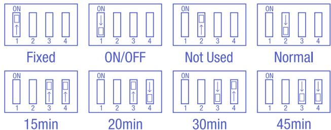
Note: switch number 2 must be set off (down) Normal. If switch 2 is set on the timer will only run for 1 minute.
